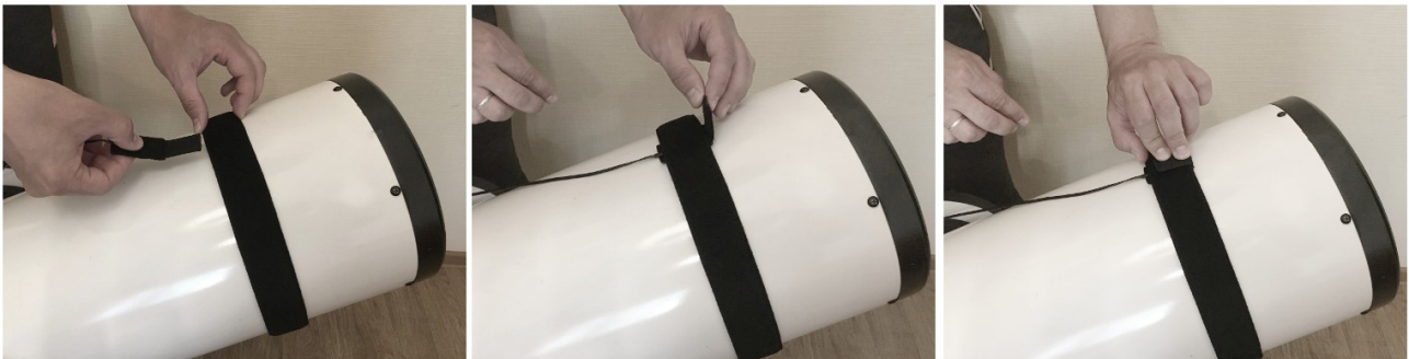
Figure 3 EXAMPLE. Telescope temperature sensor installed on refractor (SCT or MAC).
